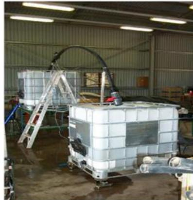
Figure 1 Flow meter evaluation System
