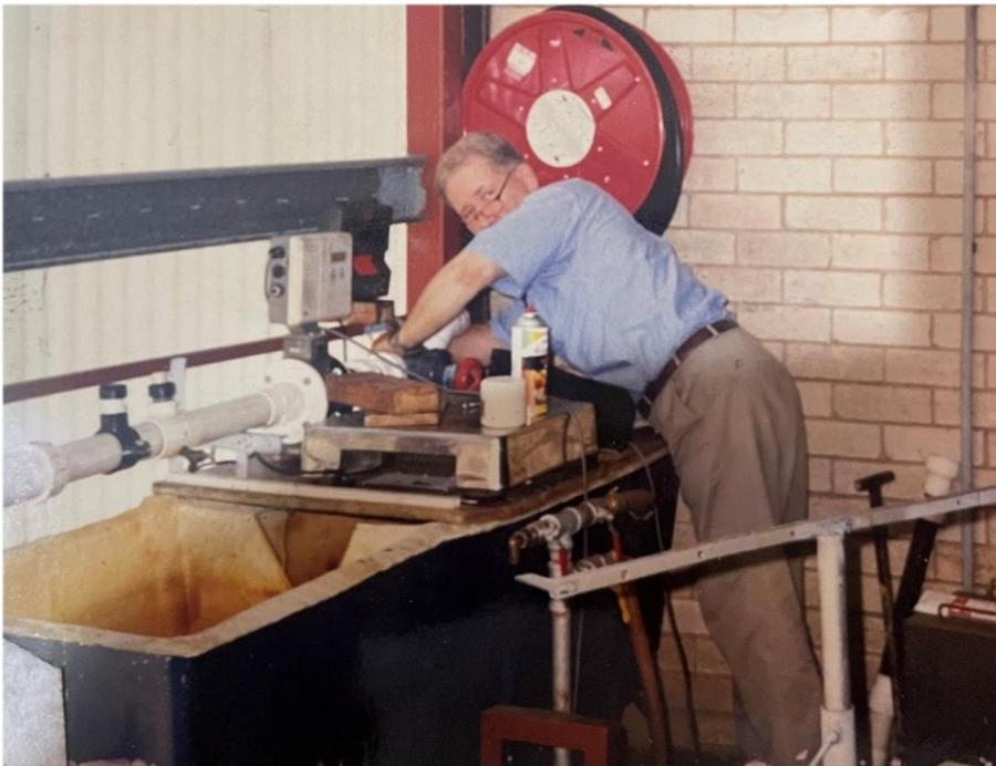
Tony pictured setting up re-plumbing the famous Flowmeter Testing Flow-Rig with Mag-Master flowmeter and wiring the load cell verifying equipment.
