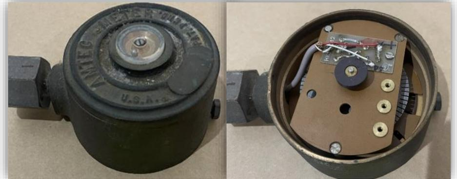
(Above) Manu converted high-resolution optical pulse head for Amtec Flowmeter and (Below) Carlon/Manu USA Flowmeter.
