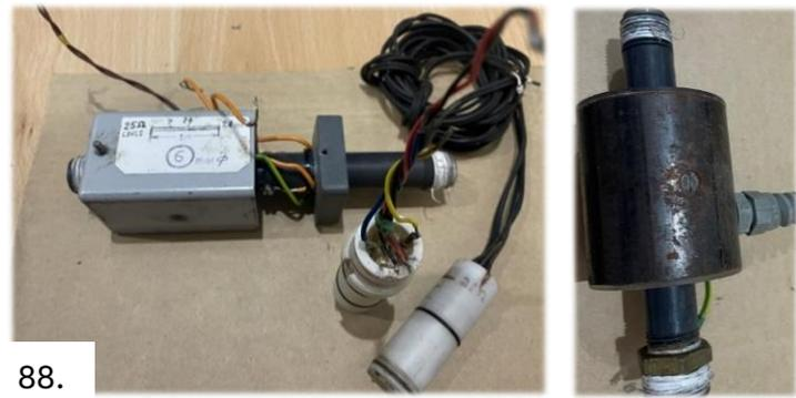
◀ Original Full bore 15mm flow-tubes and insertion types.
