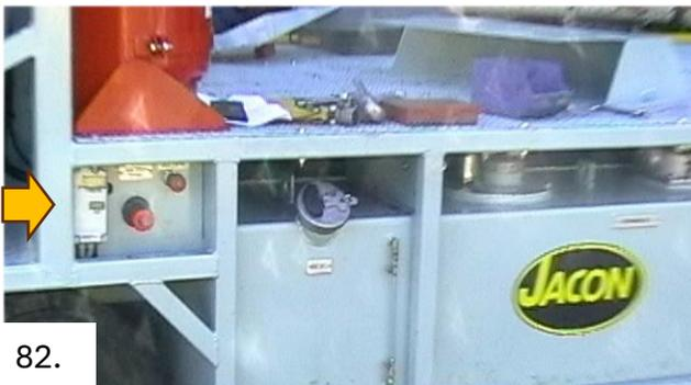
▲ Shotcrete spray-rig with Manu flowmeter installed.
